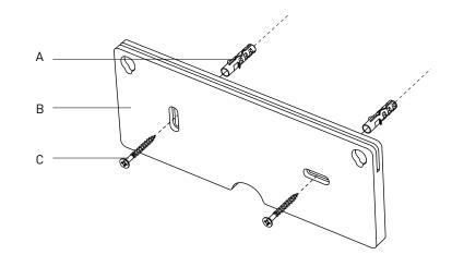
STEP 1: Attach the wall mount (B) onto the wall with the delivered
