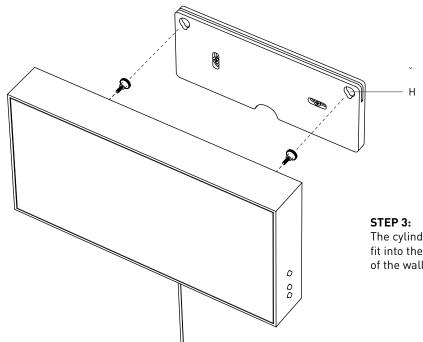
The cylinder head screws fit into the holes (H) of the wall mount.
