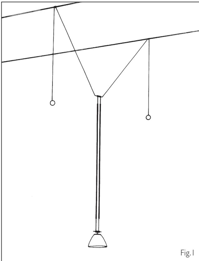
Hang the shade between the current-bearing cables of your YaYaHo system and drape the wires with the counterweights over the cables. (Fig. 1)
